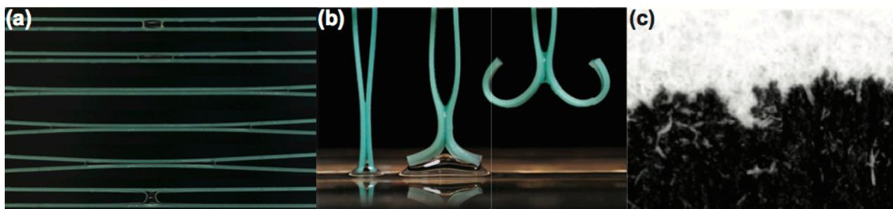
*Fig: Model experiment on (a) the wetting of flexible fibers and (b) the swelling of elastomeric plates. (c) imbibition front in paper.*
