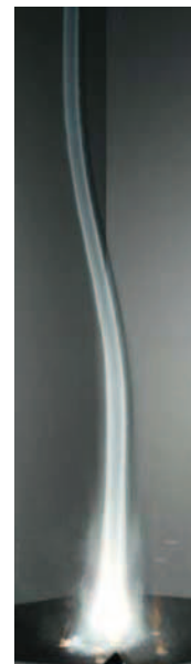
Fig. 2. "Tornado apprivoisée" a 3m high open tornado simulator. (© Jean-Marc Chomaz)
